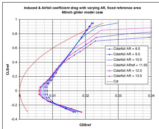
Nevertheless a notable fact is related to the lower Reynolds number band [100 000 – 500 000] the airfoil is functioning in : the variation of airfoil drag with chord (in “true” aerodynamic coefficient) is much steeper that for full size standard class glider.
