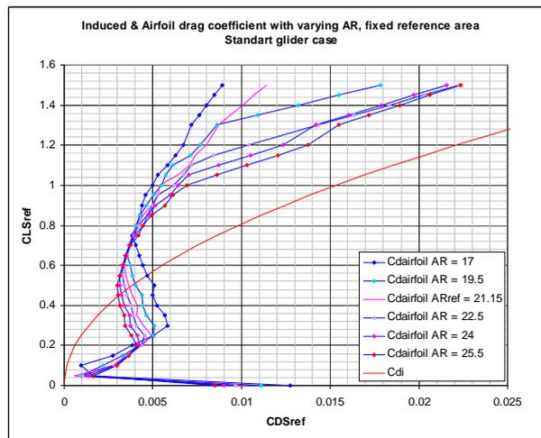
For a given speed, induced  $CD_{Sref}$  is virtually constant over the different homothetic wings (already detailed) : then very dependency to AR / area comes from the airfoil drag. The conclusion drawn here means that a driving factor when considering speed polar is related to area : less area of wing leads to less airfoil drag at low  $CL_{Sref}$  thanks to less wetted area.
