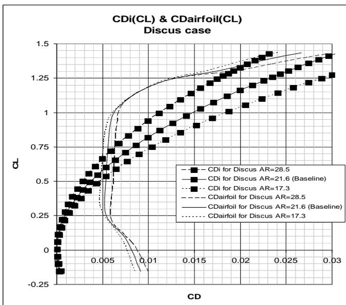
**Figure 9 :** Wing drag split, for various plan-form.
