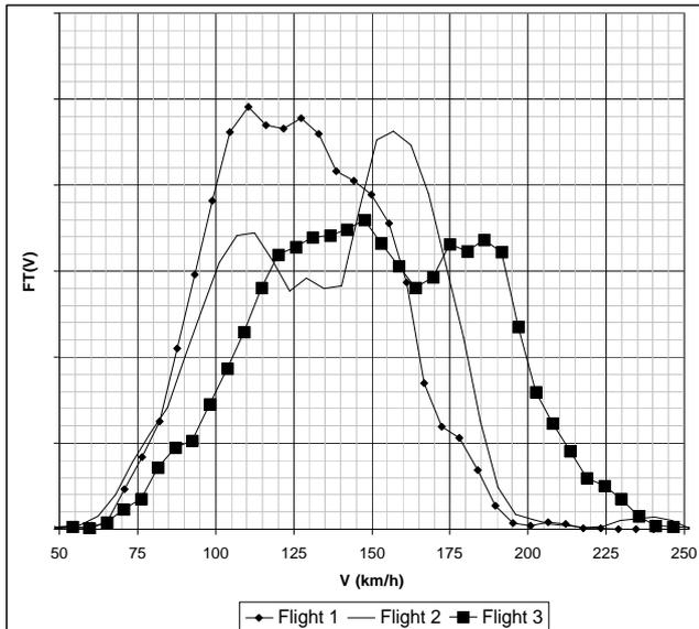
Figure 1 : Speed spectrum for the three detailed flights.
