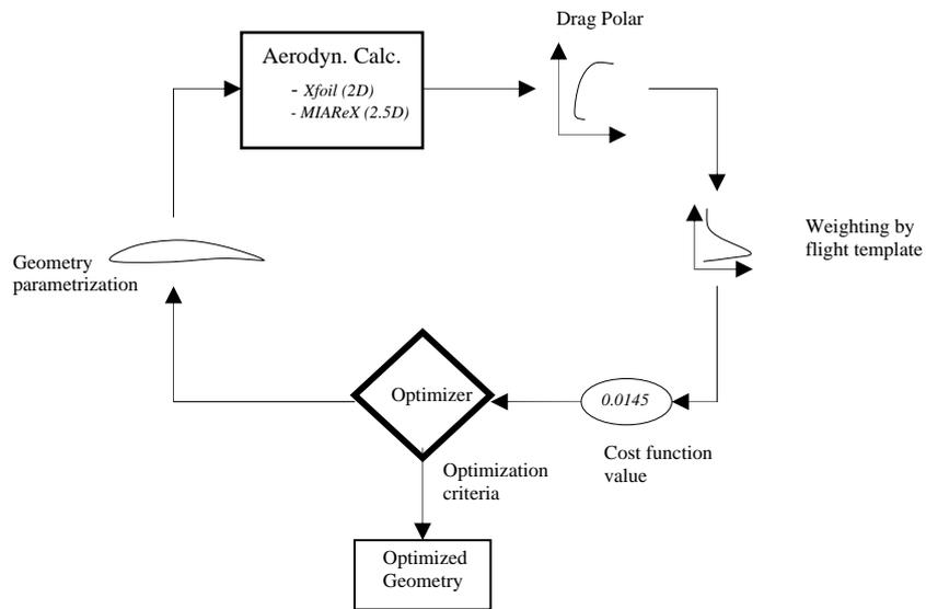
**Figure 11 :** Numerical optimization process scheme.
