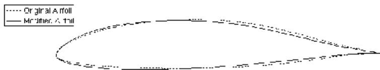
**Figure 12 :** Airfoil geometry resulting from numerical optimization.
