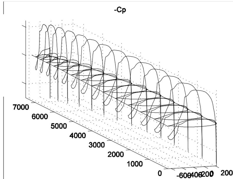
**Figure 8 :** The extended Lifting line theory computes local behavior of each airfoil, and induced drag.
