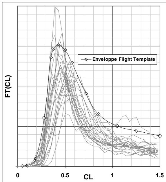
Figure 3 : Envelope flight template
