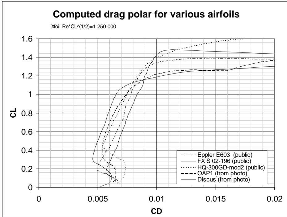
**Figure 4 :** Calculated drag polars for five samples airfoils
