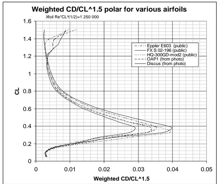
**Figure 6 :** Weighted  $CD/CL^{1.5}$  polars for the same five samples airfoils
