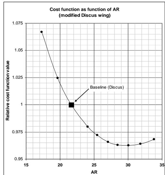
**Figure 10 :** Aerodynamic AR optimum, according to criteria derived from Flight template.
