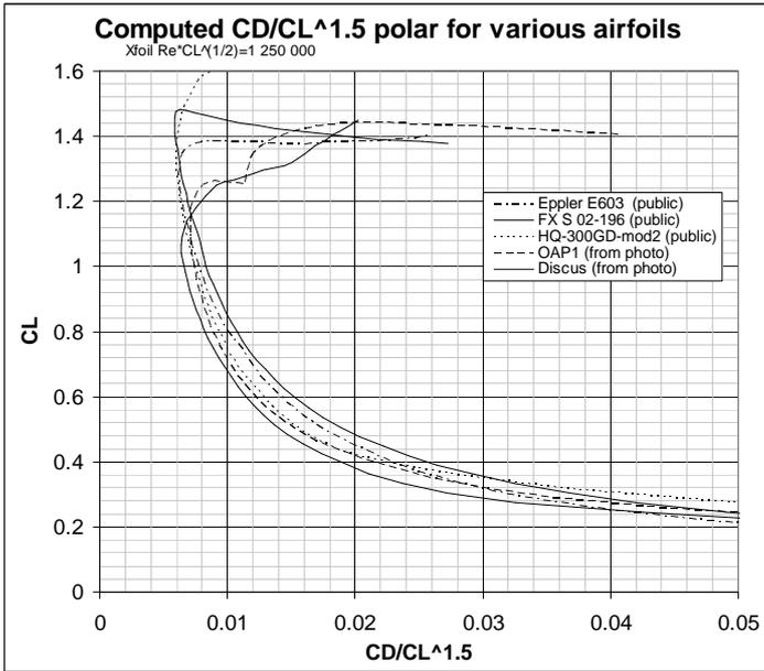
**Figure 5 :** Calculated  $CD/CL^{1.5}$  polars for the same five samples airfoils
